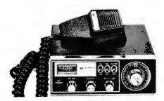
er features include: a PA switch that delivers 3 watts of audio power, a warning light that indicates antenna mismatch or failure; an S/r-f meter, and an external CB switch that directs received CB signals to an external speaker.
